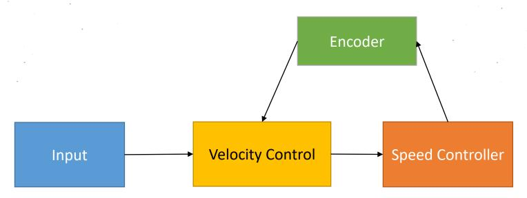
This year, we have implemented a PID-based velocity control algorithm.
